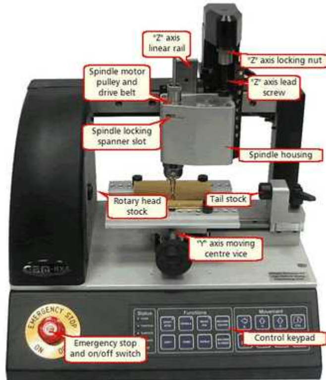
The front view of the GEM-RX4 Engraving Machine showing the main controls.
